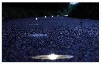
Figure 23: Example of a foot/cycle path which is lit by solar cat's-eye providing some light for pedestrian and cyclists without creating any disturbance to the nearby properties or unacceptable levels of light pollution.
